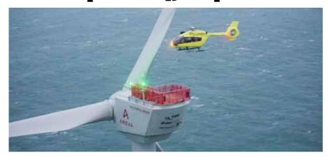
Airbus has extended the flight envelope of the H145 by improving the helicopter's "One-engine-inoperative" (OEI) power. OEI evaluates the performance of an aircraft with only one engine functioning. The light-twin helicopter H145 can now house two other technicians or can fly longer distances during a mission which requires human external cargo (HEC) operations.
