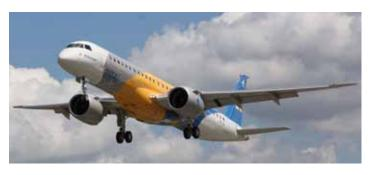
"With 1.4 meters longer wingspan than the E190-E2, the E195-E2 becomes the aircraft with the highest aspect ratio among single-aisle jets thus increasing fuel efficiency" said Luís Carlos Affonso, COO, Embraer Commercial Aviation. "We also applied experience from over 17 million hours of flight and 100 jet airline customers to develop the E195-E2 with the most competitive life cycle cost in the industry."
