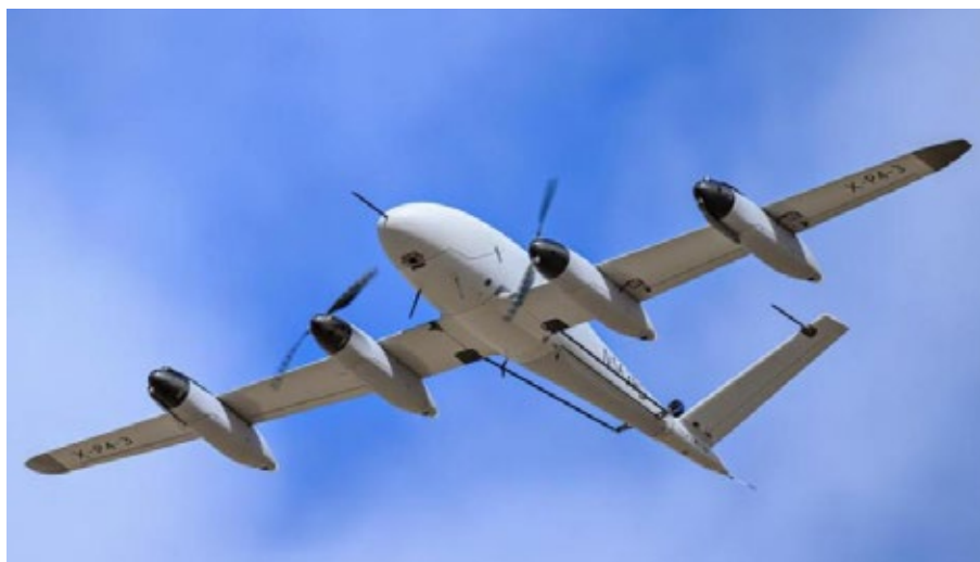
■ PteroDynamics's Transwing is a pioneering VTOL aircraft that merges fixed-wing speed, range, and endurance with superior VTOL performance.
